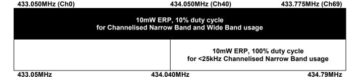
433.050-434.790 MHz, Non Specific Short Range Device, band is primarily intended for Telemetry, Telecommand, Alarms, Data in general and other similar applications. Audio and Voice signals should be avoided in the band.
