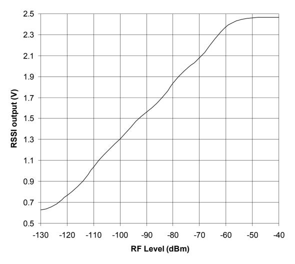
Figure 5: RSSI voltage variation with respect to RF level at TR2M
