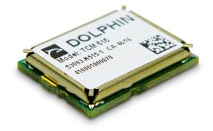
ESP3 messages received from the external host will be encrypted and authenticated as required and then transmitted as EnOcean radio telegrams.
