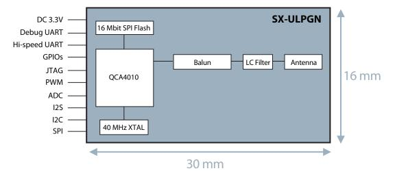
SX-ULPGN is based on the QCA4010 Reference Hardware & Software. The Software and documentation is available on the Qualcomm Developer Network: https://developer.qualcomm.com/hardware/qca4010
