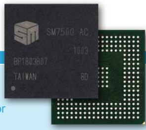
The SM750 is a PCI Express 2D multimedia mobile display controller device, packaged in a 265-pin BGA. Designed to complement needs for the embedded industry, it provides video and 2D capability. To help reduce system costs, it supports a wide variety of I/O, including analog RGB and digital LCD Panel interfaces, two Zoom Video interfaces, and Pulse Width Modulation (PWM). There are additional GPIO bits that can be used to interface to external devices as well.
