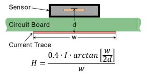
where the magnetic field H is in millitesla, the width of the trace w in mm, and d in mm. The AG905-06 produces 0.023 mT/amp at the sensor, which corresponds to  $\pm 220$  amps in the sensor's highly linear  $\pm 5$  mT range.
