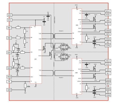
The 2SC0635T2A0-45 combines a complete twochannel driver core with all components required for driving, such as an isolated DC/DC converter, short-circuit protection, Advanced Active Clamping as well as supply voltage monitoring. Each of the two output channels is electrically isolated from the primary side and from the other secondary channel.
