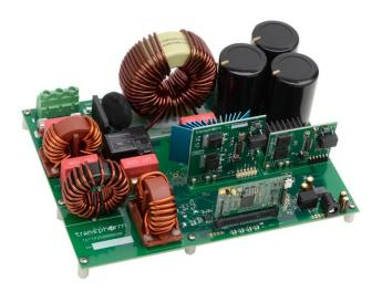
Figure 1. TDTTP2500B066B 2.5kW totem-pole PFC evaluation board
