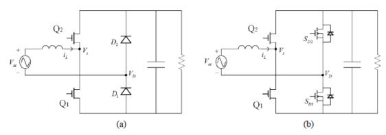
Fig.3 Totem-pole bridgeless PFC boost converter based on GaN FET (a) Diode for line rectification (b) MOSFET for line rectification
