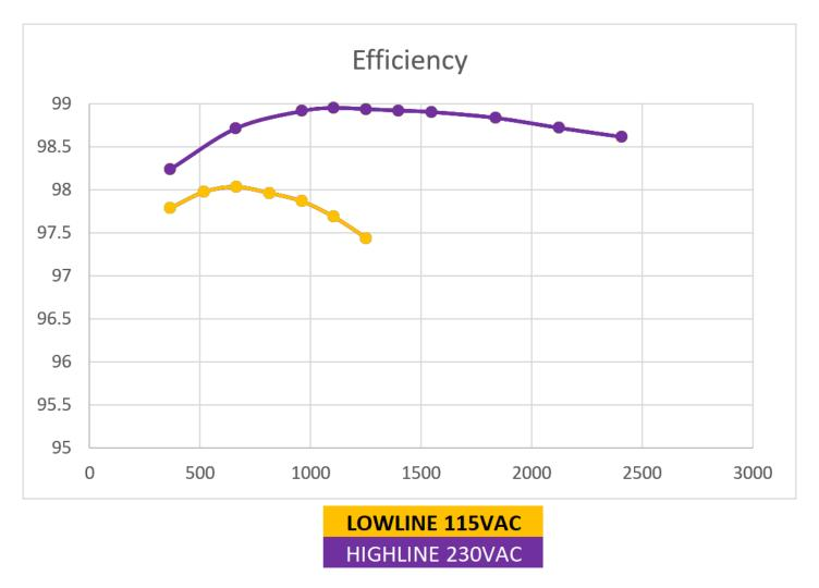
Figure 16. The efficiency results for Bridge-less Totem-pole PFC Evaluation Board.
