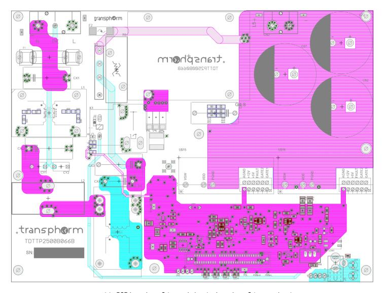
(c) PCB inner layer 2 (ground plane) + inner layer 3 (power plane)
