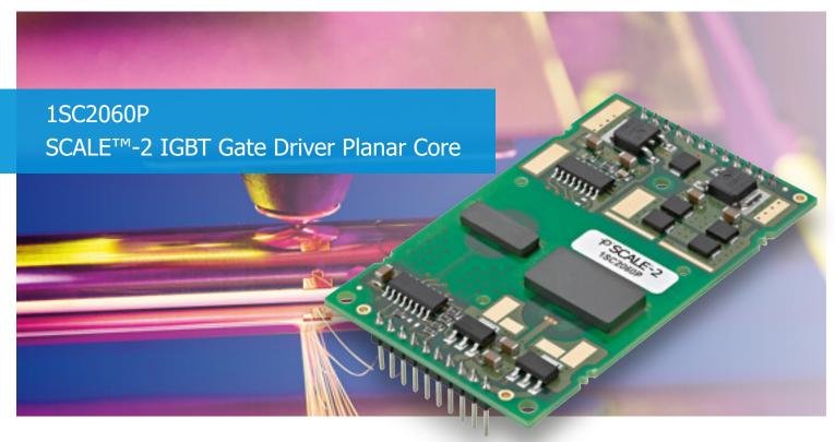
1SC2060P – Single-Channel Gate Driver Core with 60 A Gate Current for Driving Large IGBT Modules in Parallel 20 W Output Power for High-Frequency Applications up to 500 kHz.
