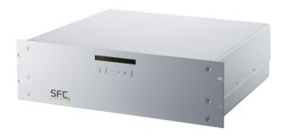
21 kW, water cooled, for DC and pulsed applications, 3 phase mains (no neutral), up to 12 channels current/voltage source. Rise/fall times less than 50  $\mu s$ . Safety interlock, PLe
