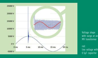
According to a study published on an IEEE-conference in 1995, the additional cost and space spent on surge capacitors are well worth the extra expense (approx. 15 - 20% of the motor cost): an alternative over-sizing of the initial motor or transformer windings for enhanced strength against transient over-voltages would require a bigger winding window which would imply a larger machine and a cost increase by approx. 35...50%.
