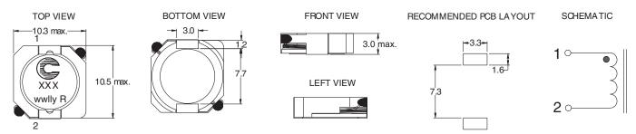
Dimensions are in millimeters.
