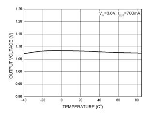
Fig. 7 Output Voltage vs. Temperature
