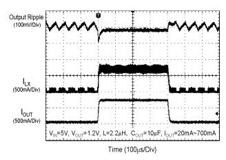
Fig. 14 Load Transient Response
