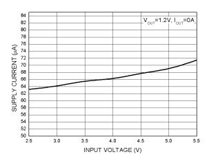
Fig. 11 Supply Current vs. Input Voltage
