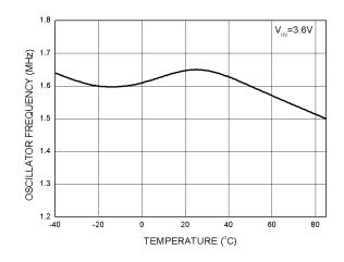
Fig. 8 Oscillator Frequency vs. Temperature
