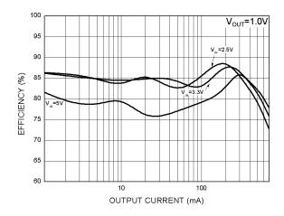
Fig. 4 Efficiency vs. Output Current
