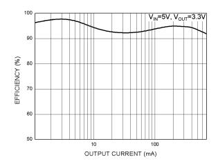
Fig. 6 Efficiency vs. Output Current
