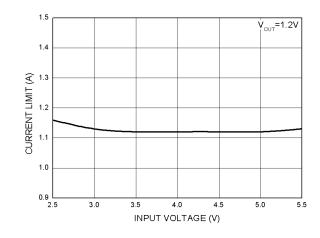
Fig. 12 Current Limit vs. Input Voltage
