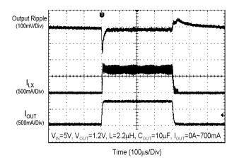
Fig. 13 Load Transient Response
