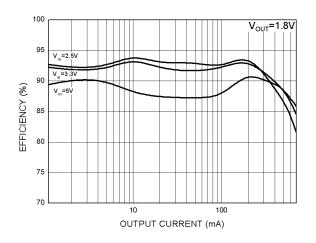
Fig. 5 Efficiency vs. Output Current
