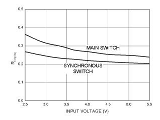
Fig. 10 R<sub>DS(ON)</sub> vs. Input Voltage
