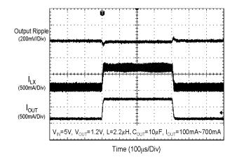
Fig. 15 Load Transient Response
