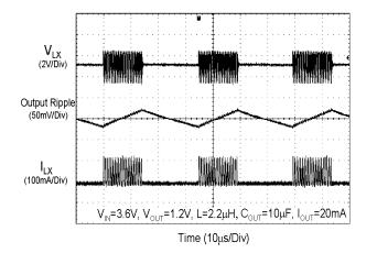
Fig. 17 PSM Operation
