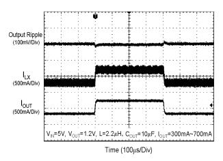
Fig. 15 Load Transient Response
