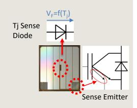
Switching speed control using the sense-emitter: An innovative switching speed control can be established depending on the actual value of the collector current I<sub>c</sub>. This means - a reduced speed (for Low EMI) turn-on at low I<sub>c</sub> values and a high speed turn-on (low turn-on loss) at high I<sub>c</sub> values can be achieved. This approach delivers a higher inverter efficiency while simultaneously ensuring good EMI performance during operation.
