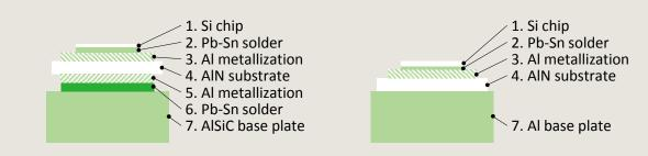
New base plate results in higher thermal conductivity between junction and case and an increased thermal-cycling performance
