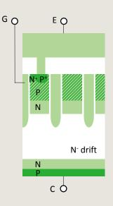
Compared to previous product<sup>\*</sup>, active chip area is increased 28 % by optimizing edge termination. \* CM750HG-130R
