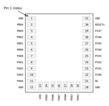
Figure 6.1. 31-Pin PCB Module With LF Crystal Device Pinout
