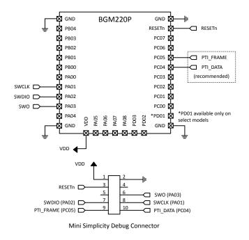
Figure 5.2. Stand-Alone SoC Configuration
