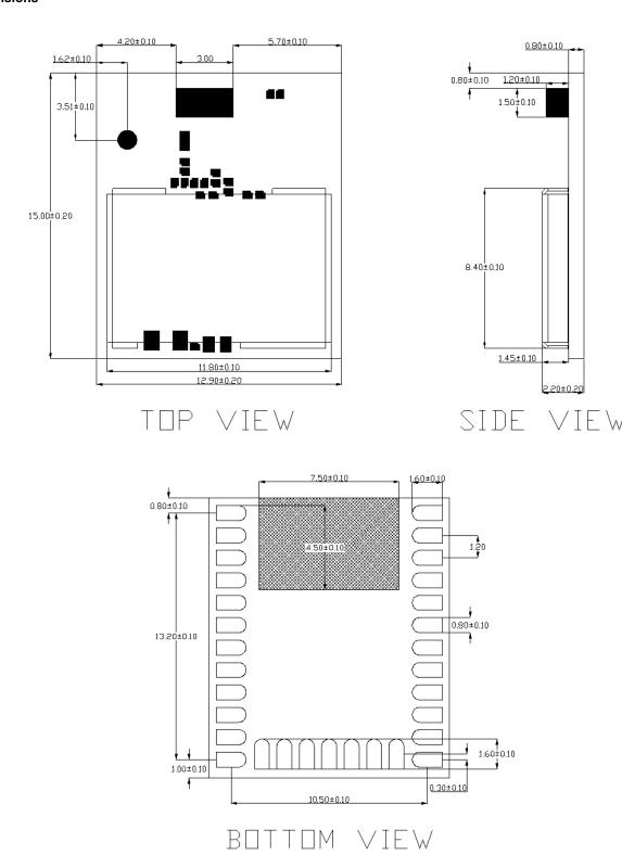
Figure 8.1. Module Dimensions
