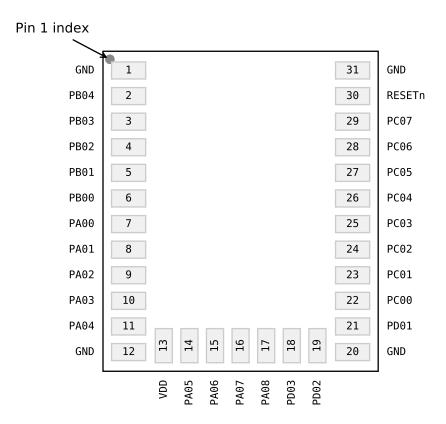
Figure 6.2. 31-Pin PCB Module With Precision LFRCO Device Pinout
