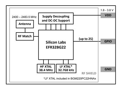
Figure 3.1. BGM220P Block Diagram
