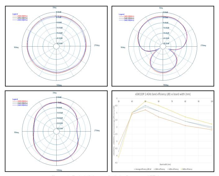
Figure 4.3. Typical 2D Antenna Radiation Patterns and Efficiency
