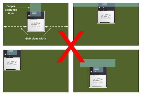
Figure 7.2. Non-Optimal Layout Examples
