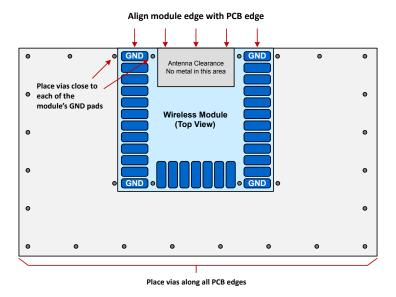
Figure 7.1. Recommended Layout for BGM220P
