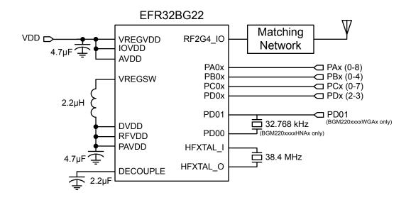
Figure 3.2. BGM220P Module Schematic
