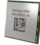
Wi-Fi 5 and Bluetooth v5.2 embeddable SiP
