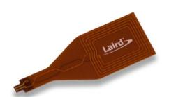
This NFC flex PCB antenna is included with the DVK-BL6xx products. It was tested with the BL65xx series of modules for NFC applications and use.
