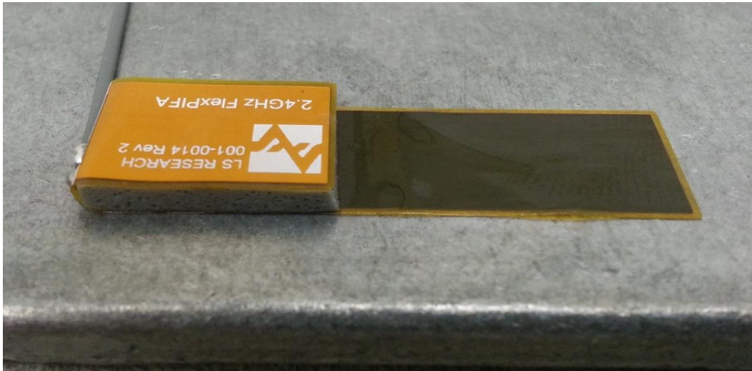
Figure 25: FlexPIFA mounted on metal
