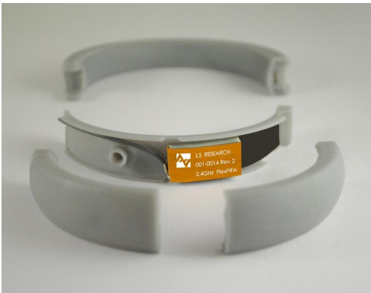
Figure 28: FlexPIFA integrated into bracelet
