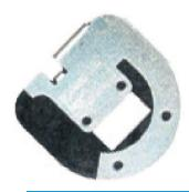
Laird's D-Puck antenna is a cost-effective, small-scale metal antenna designed for maximum durability. This vertically polarized antenna has a gain of >3 dBi at 2.4-2.5 GHz and >4 dBi at 5.15-5.875 GHz. The D-Puck is specifically designed to be embedded inside devices for aesthetically pleasing integration with high durability.
