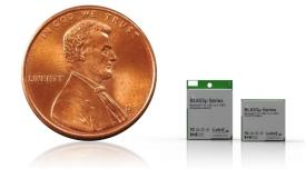
Laird Connectivity's latest range of Nordic nRF52833 based modules specifically targets OEMs where space is constrained in their designs. Yet still the miniaturized BL653µ series enables Industrial OEMs to robustly implement longer range Bluetooth Low Energy (LE) applications in the harshest operating environments. This series of secure, low power microcontroller modules with multi wireless capabilities is the future of wireless Internet of Things (IoT) connectivity.
