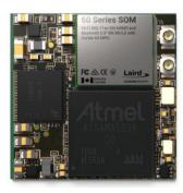
Laird Connectivity's 60 Series SOM brings all of Laird Connectivity's industry competence and capabilities into one solution. The SOM provides superior enterprise-class Wi-Fi connectivity with full support for 2x2 MIMO 802.11ac WLAN, plus Bluetooth 5.1 dual-mode. This solution is equipped with a Cortex A5 applications processor, wireless and wired connectivity, enterprise-grade security, LCD support, and comprehensive Linux board support package (BSP).
