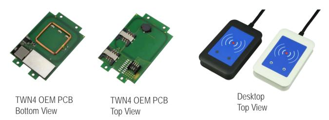
Elatec's family of TWN4 transponder readers/writers allows users to read and write to almost any 125kHz, 134.2kHz and 13.56MHz tags and/or labels. It supports all major transponders from various suppliers like ATMEL, EM, ST, NXP, TI, HID etc. and ISO standards like ISO14443A, ISO14443B, ISO15693, ISO18092 / ECMA-340 (NFC).
