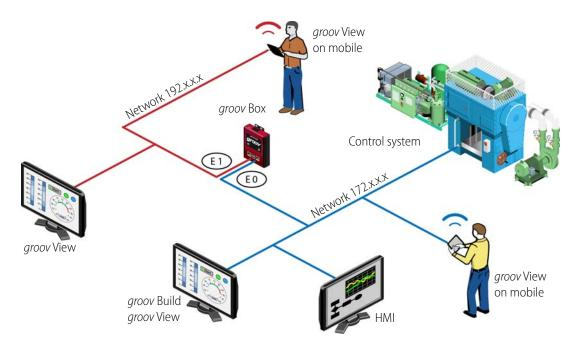
In this example, your *groov* Box is connected to your company computer network using Eth1 and to your control network using Eth0. (You could do the same thing with *groov* Server for Windows running on a PC that has two network interface cards.)
