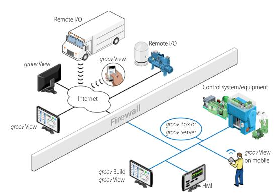
Any two networks can be used as long as both are connected to the Internet:
