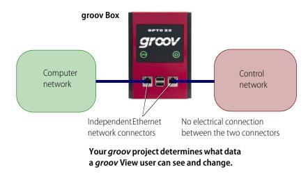
**Remember:** The independent network interfaces on *groov* Boxes must always be on separate networks (using different IP addresses and subnet masks). *groov* Boxes do not route IP traffic; they have no routing tables or network address translation. There is no communication between the two networks.
