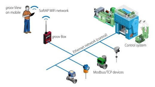
Again, the mobile devices on the SoftAP WiFi network have no direct connection with the automation equipment on the control network. Authorized employees on mobile devices who join the SoftAP network can see only the data and controls you've built into the *groov* interface.
