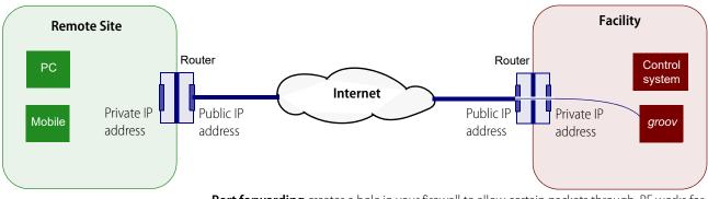
**Port forwarding** creates a hole in your firewall to allow certain packets through. PF works for *groov* because *groov* provides encryption and requires authentication from all users.
