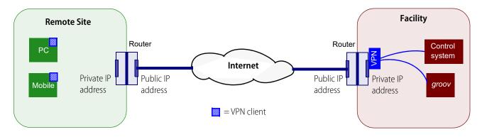
NOTE: In our diagram we're assuming that the control system and groov are at the same location. If they're not, and you need to have groov communicate with a remote PAC? For this scenario, see "VPN special case" on page 24.
