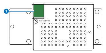
1 CAT5e/6/7 IN: Connect to the Transmitter unit with CAT5e/6/7 cable for transmission of all data signals.
