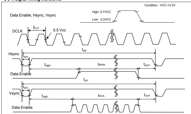
Notes: VCC means logic power voltage. (typ. 3.3V)
