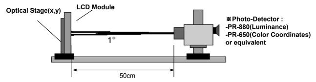
FIG. 3 Electro-optical Characteristic Measurement Equipment and Method
